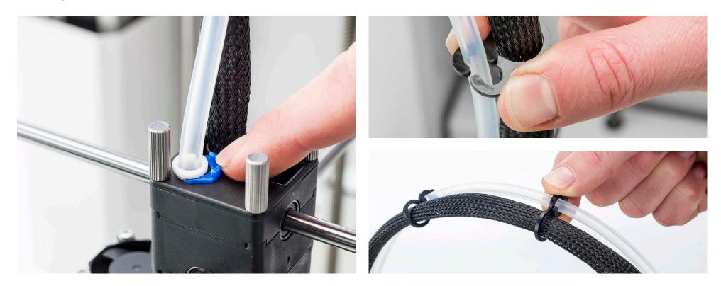
5. Secure the clamp clipPlace the blue clamp clip around the tube coupling collet to secure the Bowden tube.
